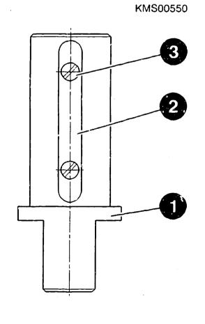
Clamping pin for drive spindle with multi-plate clutch
